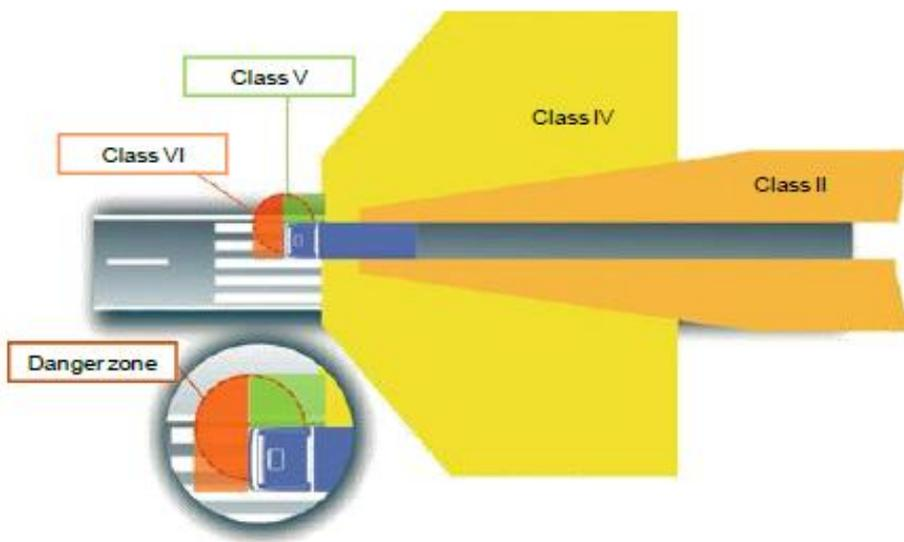
Figure 3: Field of vision requirements 2003/97/EC<sup>11</sup>
