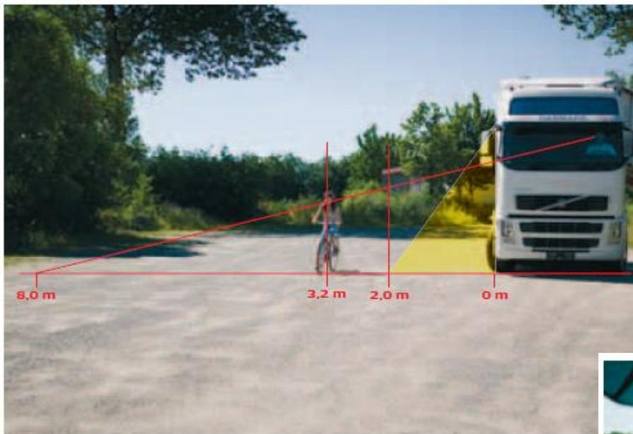
Figures 6: Distance to side of vehicle, necessary for cyclist to be seen directly by driver
