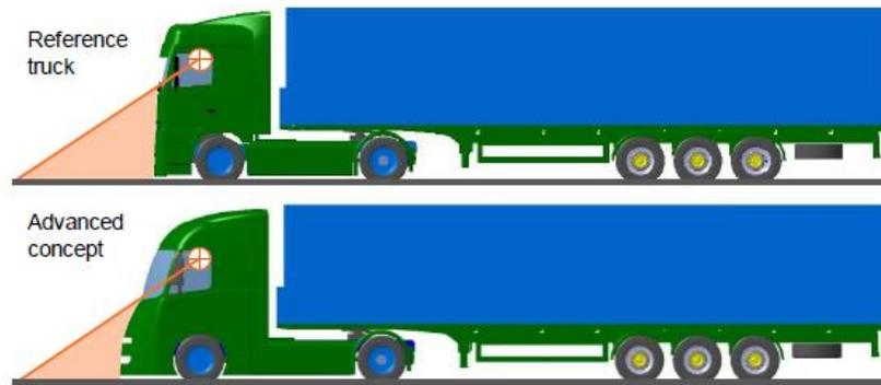
Figure 9: Direct visibility through front screen<sup>20</sup>
