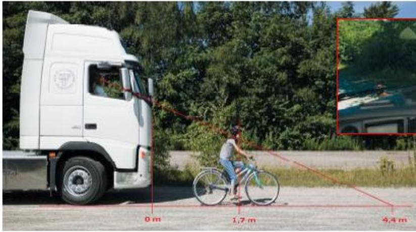
Figures 5: Distance in front of vehicle, necessary for cyclist to be seen directly by driver and the view from the cab, showing little leeway for error<sup>13</sup>
