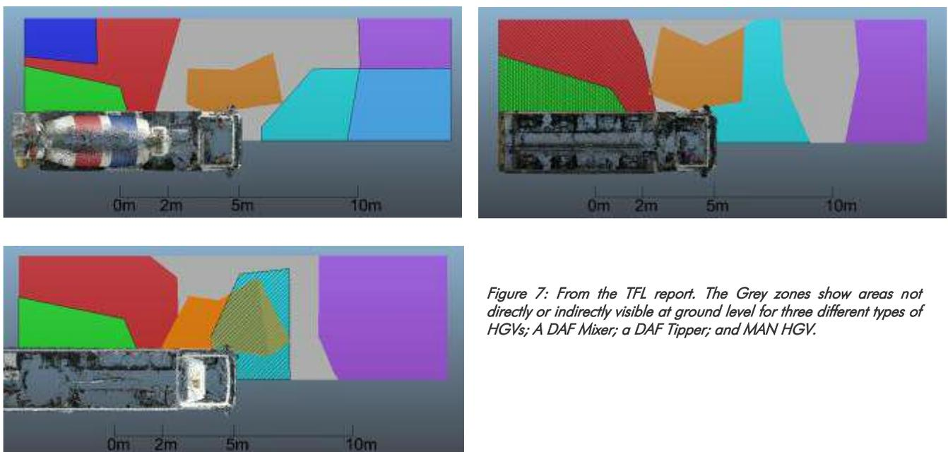
Figure 7: From the TFL report. The Grey zones show areas not directly or indirectly visible at ground level for three different types of HGVs; A DAF Mixer; a DAF Tipper; and MAN HGV.
