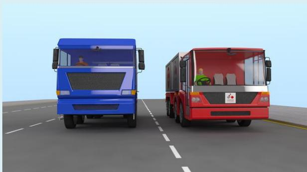
*Figure 12; comparison between a traditional construction HGV and its possible redesign with lower, better placed cab<sup>23</sup>*
