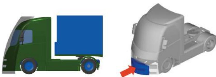
Figure 8: round nose cab with crash management system (crumple zone)<sup>19</sup>
