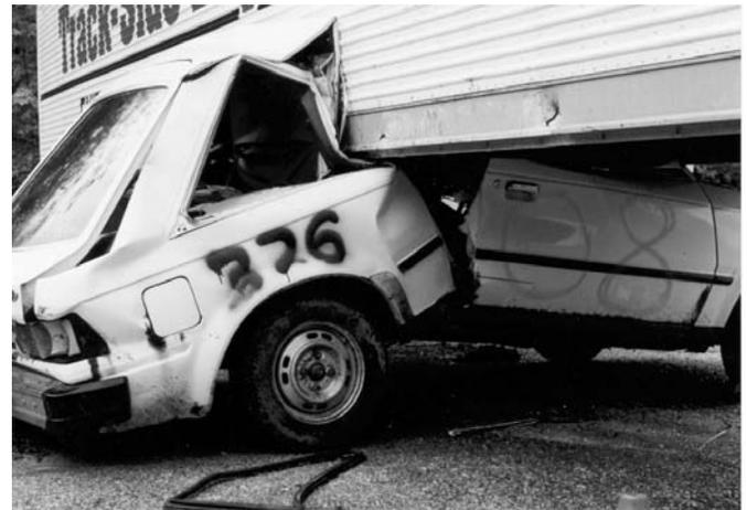
**Figure 2. 'Bend Down' Condition**
