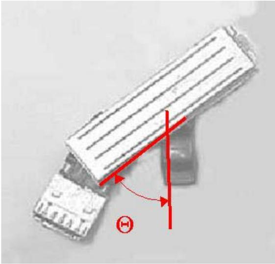
**Figure 1. Contact Angle**
