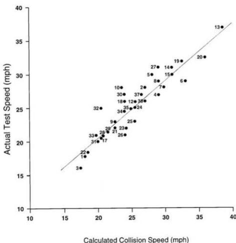
**Figure 4. Actual versus Calculated Speeds**
